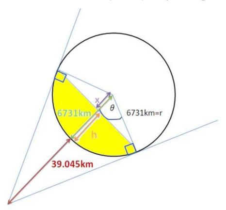
By considering his field of vision to be a spherical cap and then looking at the cross section of the earth we get the diagram shown above. Felix starts at the point where the two tangents meet and his area of vision is the part shaded in yellow. In order to find the surface area of this spherical cap we need to know the distance h.
