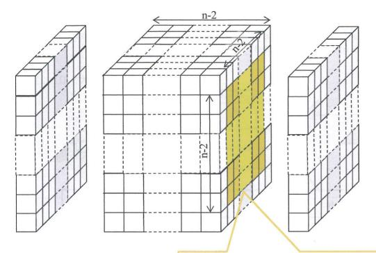
The only small cubes without any paint on them are the ones on the inside, beneath the outer layer of small cubes. These small cubes make up a cube. To get the height of this cube you must use the height of the whole cube (this dimension = n) but subtract 2 from it to get rid of the outer layer of small cubes. All you then have to do is cube it to get the number of small cubes in this middle cube.
